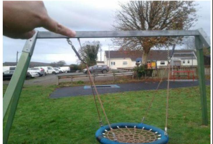
**Finding:** The shackle links are worn in excess of 40% and require renewing ( the shackle is wearing due to the length of the secondary safety chain taking all the weight of the basket instead of the main suspension
